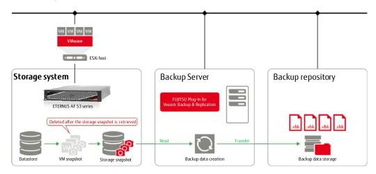
Figure 4-2 Linkage to Veeam Backup & Replication with Veeam Plug-In
