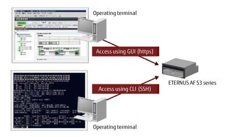
Figure 5-5 Strengthened Security with SSL/SSH
