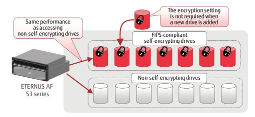
Figure 5-6 Preventing Information Leakage using Data Encryption
