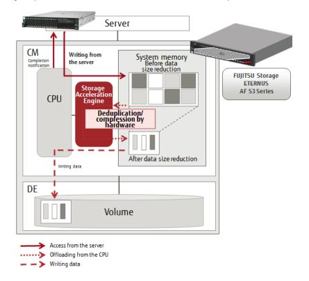
Figure 3-1 CPU Offloading to the Storage Acceleration Engine during Data Compression
