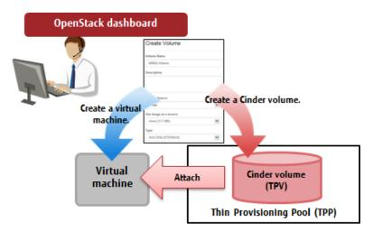
Figure 5-8 Operation of the OpenStack Dashboard
