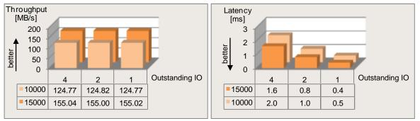
Standard load profile "Streaming" (sequential access, 100% read, 64 kB block size)
