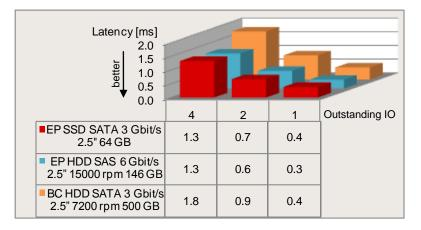
With restore the throughput of the SAS-HDD is just under 40% higher than that of the SATA-HDD, the response times are just under 30% lower. In comparison with the SAS-HDD, the throughput and response times of the SATA-SSD are slightly worse.
