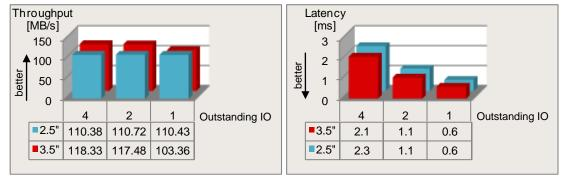
Whereas the 3.5" hard disk with the standard load profiles and with sequential access provides a higher throughput than the 2.5" hard disk, the 2.5" hard disk with standard load profiles and with random access is at the forefront. However, this example cannot be generalized.
