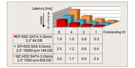
With streaming the throughput of the SAS-HDD is about 40% higher than that of the SATA-HDD. Compared with the SAS-HDD, the SATA-SSD offers a higher throughput of about 30%. The response times are reduced by about 20% - 30% in each case.
