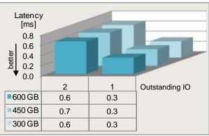
The following ten diagrams show performance values (transactions, throughput rates and response times) for the standard load profiles "File server", "Database", "File copy", "Streaming" and "Restore" with increasing loads through the number of parallel requests (outstanding IO). The following actual hard disks are considered
