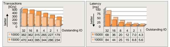
With the random load profile "File Server" the faster rotating hard disk for low load intensities (1 outstanding IO) has a performance advantage of 31%. The advantage is reduced to 23% for higher load intensities (32 outstanding IOs).
