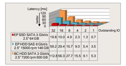
With a low load the SAS-HDD offers 50% higher transaction rates for the three standard load profiles with random access than the SATA-HDD. With higher loads the SAS-HDD provides about twice the performance of the SATA-HDD. If the load on the SAS-HDD is twice as high as that on the SATA-HDD, the response times are approximately equal.
