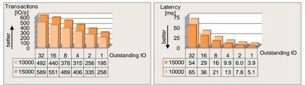
With the random load profile "Database" the faster rotating hard disk for low workload intensities (1 outstanding IO) has a performance advantage of 32%. The advantage is reduced to 20% for higher load intensities (32 outstanding IOs).
