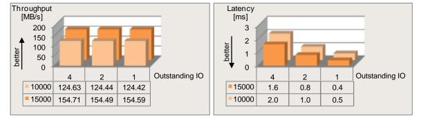
Standard load profile "Restore" (sequential access, 100% write, 64 kB block size)
