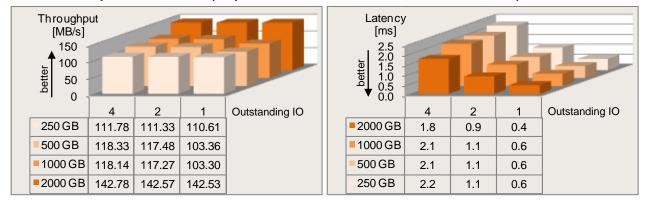
The following ten diagrams show performance values (transactions, throughput rates and response times) for the standard load profiles "File server", "Database", "File copy", "Streaming" and "Restore" with increasing loads through the number of parallel requests (outstanding IO). The following actual hard disks are considered
