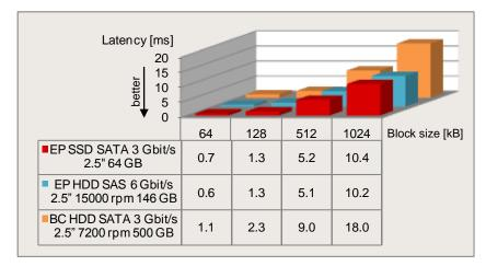
The throughput of all hard disks does not depend on block size with sequential write access. Thus, twice as high average response times and halved transaction rates are recorded with double the block size. As long as response times are of no interest, it does not matter whether an application runs with a block size of 64 kB or even larger blocks.
