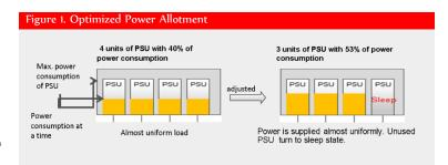
Electric equipment distributes electric power to parts inside. This is similar to water system, which provides homes with water – aging or slack of water pipes causes water leak and disturbs efficient water supply. For electric equipment, the deficiency of power consumption happens mainly in conversion or distribution of electric power. PRIMEQUEST 2000 has reduced loss of power conversion:
