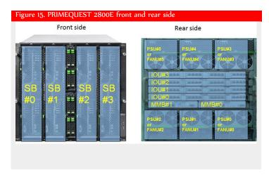
PRIMEQUEST 2000 much reduces cables because components are linked by metal board called mid plane. This means maintenance operations for PRIMEQUEST does not require cabling inside chassis. If taking off and taking on of cables were necessay, power-off of PRIMEQUEST chassis would have been necessary. So, this PRIMEQUEST design helps reduce downtime for maintenance (Figure 16)
