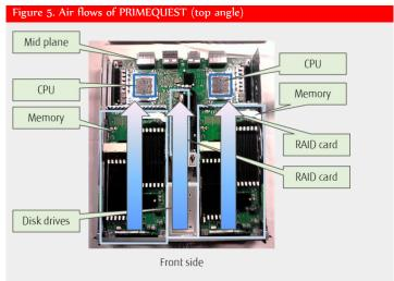
PRIMEQUEST 2000 controls fan rotational speed smoothly according to temperature changes. Former 8 socket PRIMEQUEST server controls three level of fan rotational speed. So, inefficiency of cooling was the problem because fan rotation speed tends to becomes too high, responding to a small rise of temperature. Fan control of PRIMEQUEST 2000 has much improved cooling efficiency because it respond to temperature changes in smoother way. – Small change of rotation to small change of temperature.
