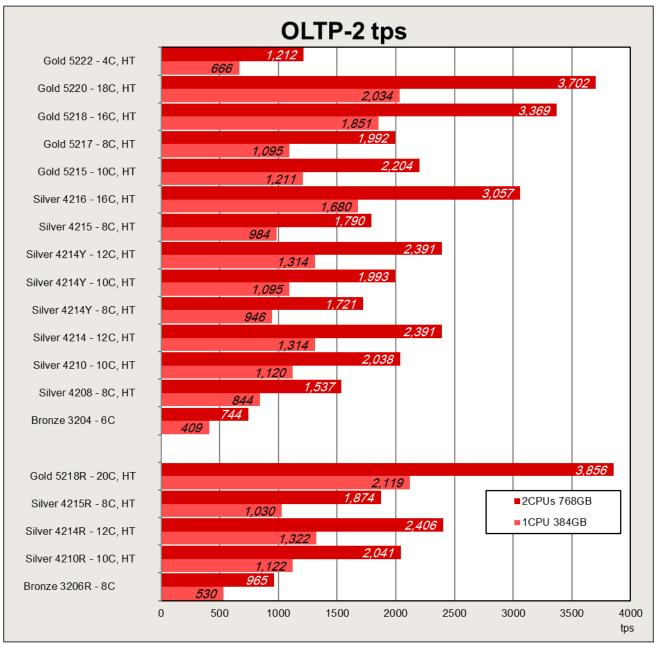
It is evident that a wide performance range is covered by a variety of released processors. If you compare the OLTP-2 value for the processor with the lowest performance (Xeon Bronze 3204) with the value for the processor with the highest performance (Xeon Platinum 8280), the result is a 5-fold increase in performance.
