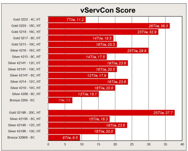
The relatively large performance differences between the processors can be explained by their features. The values scale on the basis of the number of cores, the size of the L3 cache and the CPU clock frequency and as a result of the features of Hyper-Threading and turbo mode, which are available in most processor types. Furthermore, the data transfer rate between processors ("UPI Speed") also determines performance.
