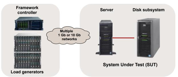
All vServCon results were Calculated based on the configuration of the next following pages of PRIMERGY RX2540 M5.
