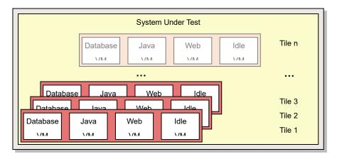
Each of the three vServCon application scenarios provides a specific benchmark result in the form of application-specific transaction rates for the respective VM. In order to derive a normalized score, the individual benchmark result for one tile is put in relation to the respective result of a reference system. The resulting relative performance value is then suitably weighted and finally added up for all VMs and tiles. The outcome is a score for this tile number.
