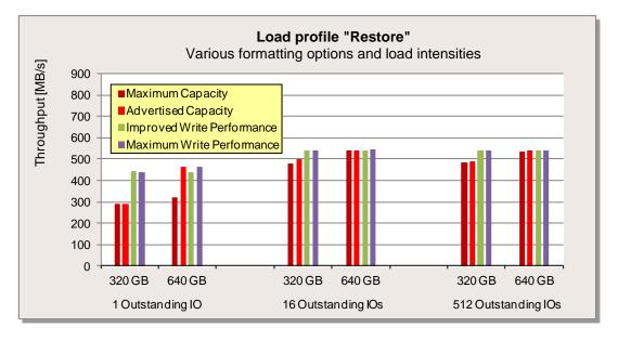
The consequence from the reduced performance differences between the various formatting options of the version with 640 GB is that reformatting from the standard formatting "Advertised Capacity" to "Improved Write Performance" or "Maximum Write Performance" is only worthwhile for random load profiles with at least 50% write share (for example with the standard load profile "File copy").
