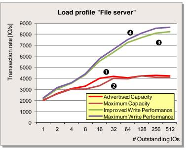
The next diagram shows the transaction rates for the "File server" load profile (random access, 67% read, 64 kB block size). In the event of "Advertised Capacity" (**0**) standard formatting and the "Maximum Capacity"
