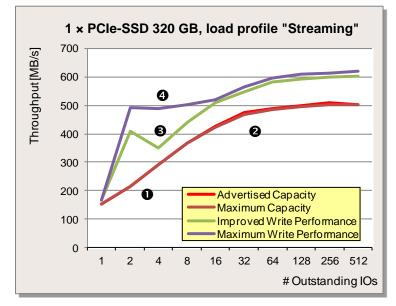
all the formatting options. If load intensity increases, the throughput for the cases of "Advertised Capacity" (**①**) and "Maximum Capacity" (**②**) increases up to about 500 MB/s. Although this is a case of pure read access, the two formatting options for increased write performance (**③④**) offer an advantage here; somewhat more than 600 MB/s can be achieved with them.
