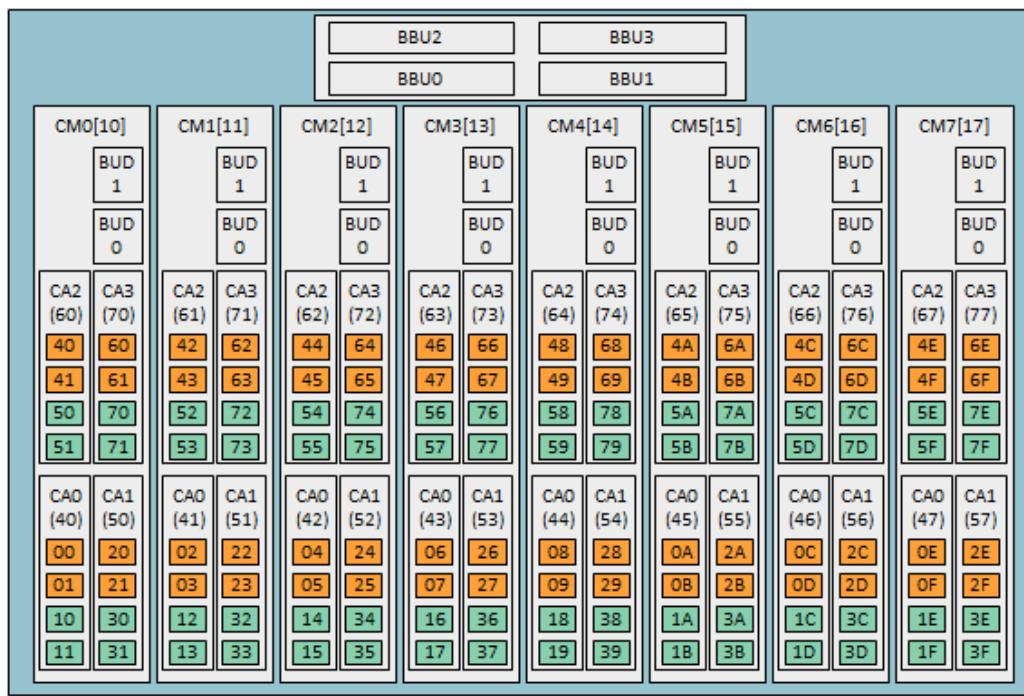
[ ]: Group No. ( ): Exchange unit No.      Orange Box : adapter Port No.      Green Box : When using 4port-CA
