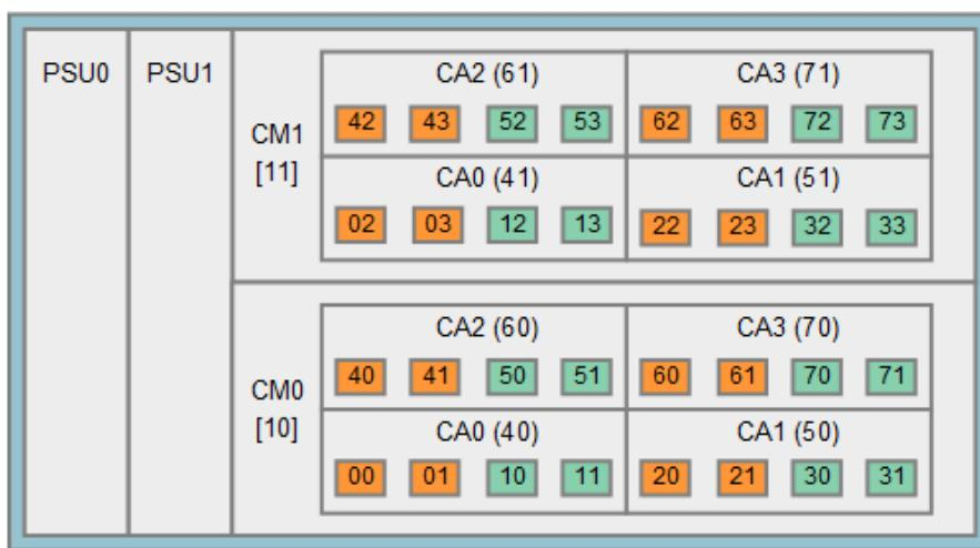
[ ]: Group No. ( ): Exchange unit No.  : adapter Port No.  : When using 4port-CA
