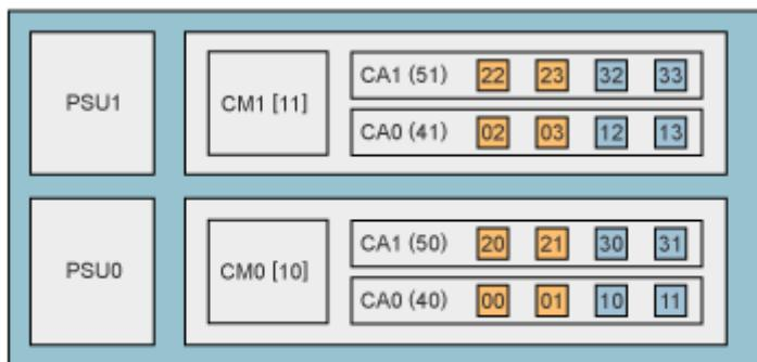
[ ]: Group No. ( ): Exchange unit No.     : Adapter Port No.     : When using 4port-CA
