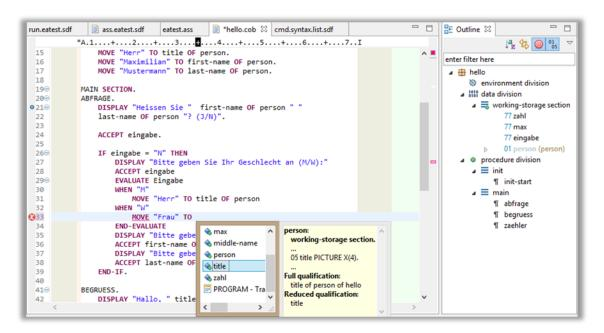
Furthermore, this editor detects a range of typical mistakes while typing and indicates those to the developer by markers similar to spell-checkers of common word processors. The input method (insert/replace) changes automatically depending on the cursor's position. By providing a Java-like Look&Feel this editor especially helps programmers of Java or similar languages to familiarize themselves with COBOL.
