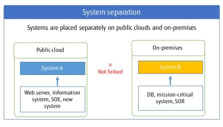
This is the most common model where different systems use different infrastructures. For example, System A is on a public cloud and System B is on-premises.
