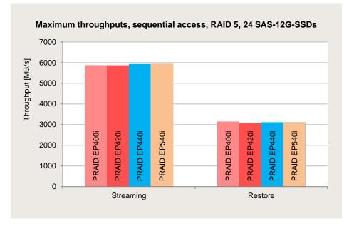
The data throughputs presented here for "Restore" (approx. 3100 MB/s) and "Streaming" (approx. 5900 MB/s) are the limits of the controllers used here for RAID 5.
