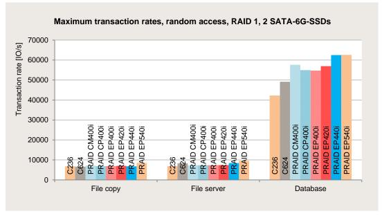
Onboard controllers improve and all controllers achieve similar performance for the standard load profiles "File copy" and "File server" but PCIe controller still has advantages for "Database".
