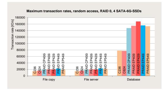
It can be clearly seen that the transaction rates are higher if the quality of the controller is higher.
