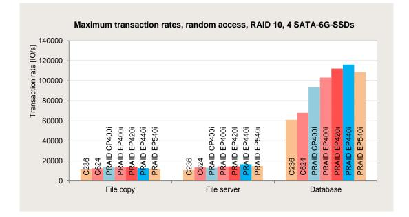
The fact that the transaction rates are higher if the quality of the controller is higher can also be clearly seen here.
