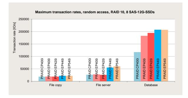
In the case of the load profile with the small blocks ("Database") the controllers with cache have an advantage here, too.
