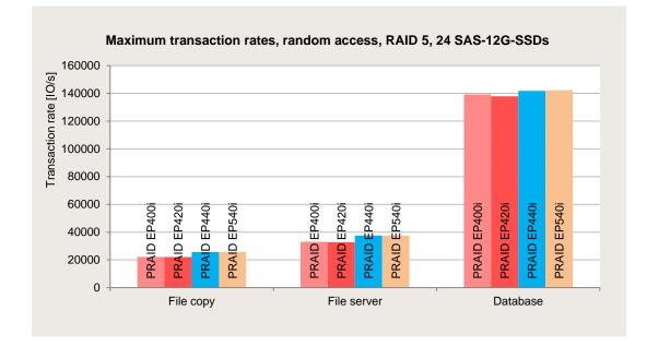
To express this in numbers of SAS-12G-SSDs, it is necessary to have between seven (8 kB block size) and 17 (64 kB block size) fully loaded SAS-12G-SSDs in order to make full use of the possibilities of the PRAID EP400i for RAID 5 - depending on the random load profile. With a smaller SSD load or other SSD types these numbers must be suitably modified.
