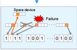
(4) Recovery of second DRAM failure The corrupted bit is corrected by ECC.
