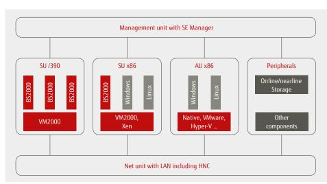
The architecture concept of the FUJITSU Server BS2000 SE series offers customers the best platform for every application scenario. The holistic management concept of the SE series considerably reduces administration and maintenance tasks, thus leading to lower costs in comparison with the operation of separate server systems.
