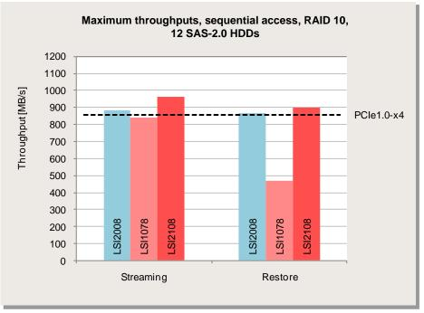
The LSI2008 and the LSI2108 controllers achieve or surpass the anticipated throughput of 930 MB/s (=  $155 \text{ MB/s} \times 6$ ) for sequential read and write.
