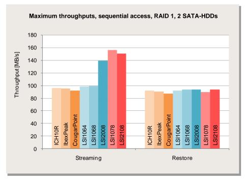
In the case of RAID 1 the controllers with a cache usually perform better if you disable the controller cache. Thus, the transaction rate of the LSI1078 and the LSI2108 controllers in this diagram are based on the following changes compared with the <u>standard settings</u> of the "Performance" mode of ServerView RAID:
