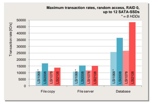
It is also interesting to understand the throughput values that are associated with these transaction rates. Despite the lower transaction rates, the two load profiles with a 64 kB block size have the higher throughputs. For example, the LSI2008 controller handles a throughput of about 1062 MB/s with the load profile "File copy".
