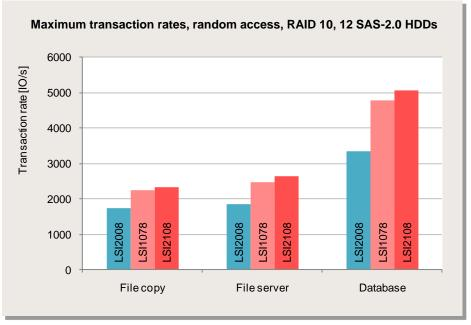
The diagram shows the same principal behavior as with RAID 0. This means that the controller without a cache (LSI2008) achieves at most about 70% of the transaction rate of the other two controllers with a cache for all the three load profiles depicted. Also for this RAID level this is a performance difference that only occurs above 32 parallel accesses to the RAID array.
