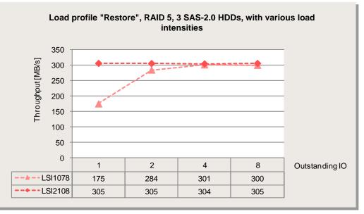
You can clearly see that in this case the LSI1078 controller does not achieve the same throughput for 1 and 2 outstanding IOs as the LSI2108 controller. The latter already achieves the maximum throughput of the RAID 5 array for 1 outstanding IO (in this case, twice the throughput of the SAS-2.0 hard disk used, i.e. 155 MB/s  $\times$  2 = 310 MB/s), whereas the LSI1078 controller only achieves a little more than half.
