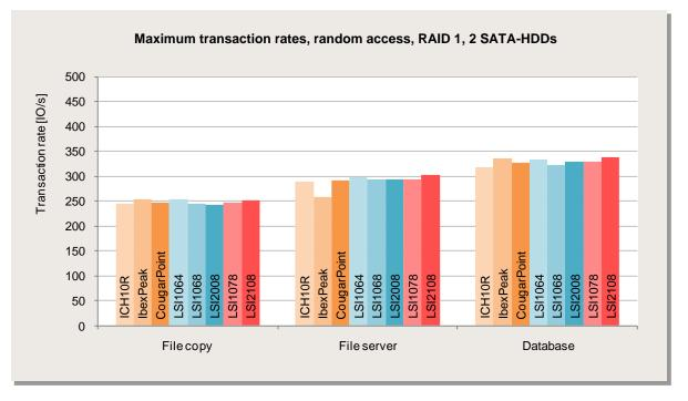
In the case of RAID 1 the controllers with a cache usually perform better if you disable the controller cache. Thus, the transaction rates of the LSI1078 and the LSI2108 controllers in this diagram are based on the following changes compared with the <u>standard settings</u> of the "Performance" mode of ServerView RAID:
