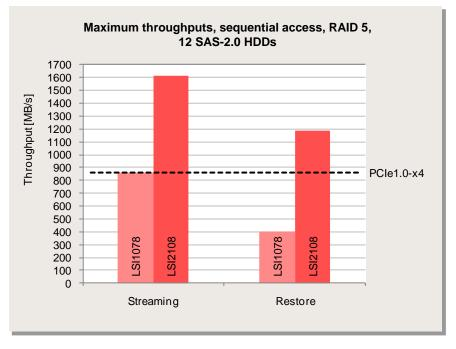
For numbers of hard disks (N) between three and twelve it is possible - as already mentioned - to estimate the throughput values to be expected for the sequential load profiles reviewed here as the (N-1)-fold value of the throughput of a single hard disk. The threshold values of the controllers cannot be exceeded here.
