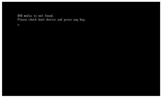
It is started from the medium of DVD/CD Drive again by connecting DVD/CD Drive while displaying the abovementioned message, inserting the medium, and inputting the key.
