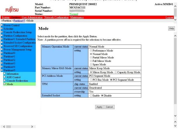
When the [Apply] button is clicked while the partition is powered on, a warning dialog box "W\_00487 Unable to change the mode, because this partition is powered on" is displayed.
