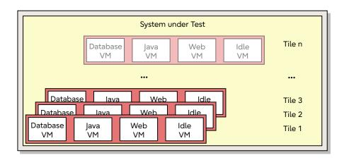
vServCon requires external load generators: exactly one client system per tile for the web server VM. Load generators and "system under test" are connected via a suitable number of networks.
