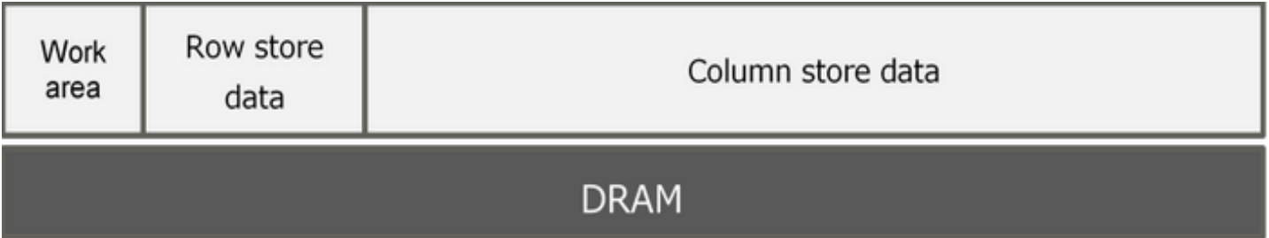
Fig. 4: Traditional DRAM memory layout and usage
