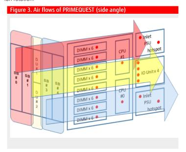
PRIMEQUEST 2000 controls fan rotational speed smoothly according to temperature changes. PRIMEQUEST 1000 server controls three level of fan rotational speed. So, inefficiency of cooling was the problem because fan rotation speed tends to becomes too high, responding to a small rise of temperature. Fan control of PRIMEQUEST 2000 has much improved cooling efficiency because it responds to temperature changes in smoother way. – Small change of rotation to small change of temperature.
