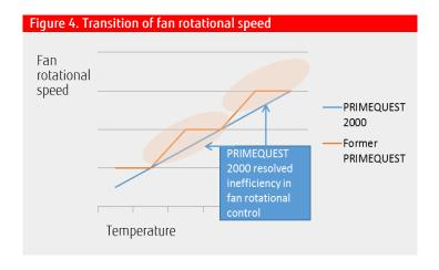
Hot spots like CPUs and memories, temperature of which rises responsively to rise of power consumption, must be cooled down by flow of cool air. Other parts, temperature of which rises less responsively to rise of power consumption, can be cooled less intensively.
