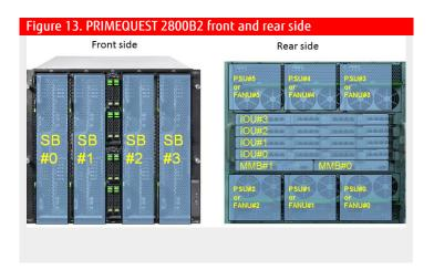
PRIMEQUEST 2000 much reduces the quantity of cables because components are linked by metal board called mid plane. This means maintenance operations for PRIMEQUEST does not require cabling inside chassis. If taking off and taking on of cables were necessay, power-off of PRIMEQUEST chassis would have been necessary. So, this PRIMEQUEST design helps reduce downtime for maintenance (Figure 14)
