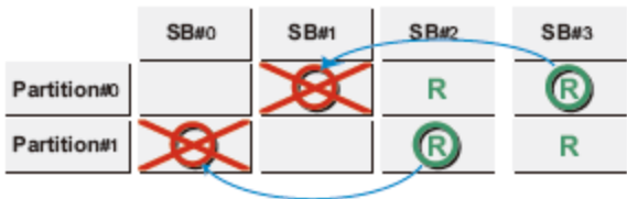
FIGURE 3.21 Example 1-b. Example when one SB is set as the Reserved SB in two partitions (SB #0 and SB #2 have simultaneously failed)
