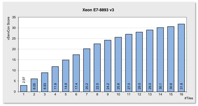
In addition to the increased number of physical cores, Hyper-Threading, which is supported by all Xeon E7 processors, is an additional reason for the high number of VMs that can be operated. As is known, a physical processor core is consequently divided into two logical cores so that the number of cores available for the hypervisor is doubled. This standard feature thus generally increases the virtualization performance of a system.
