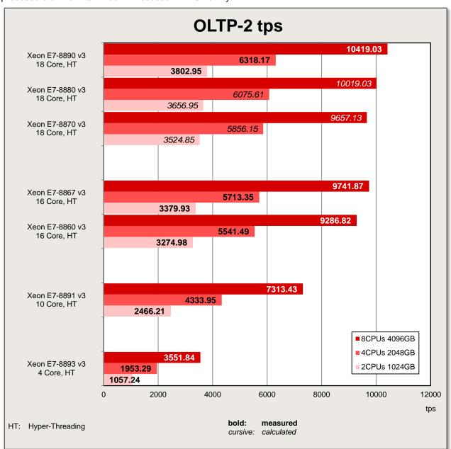
It is evident that a wide performance range is covered by the variety of released processors. If you compare the OLTP-2 value of the processor with the lowest performance (Xeon E7-8893 v3) with the value of the processor with the highest performance (Xeon E7-8890 v3), the result is a 2.9-fold increase in performance.
