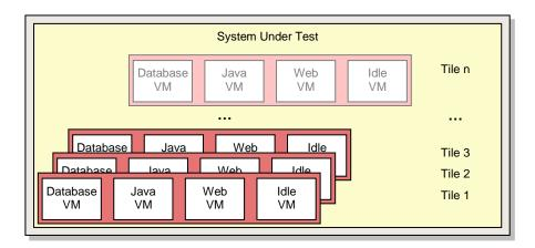
Each of the three vServCon application scenarios provides a specific benchmark result in the form of application-specific transaction rates for the respective VM. In order to derive a normalized score, the individual benchmark results for one tile are put in relation to the respective results of a reference system. The resulting relative performance values are then suitably weighted and finally added up for all VMs and tiles. The outcome is a score for this tile number.
