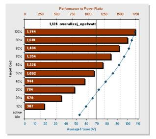
SPECpower\_ssj2008. The diagram shows a typical graph of a SPECpower\_ssj2008 result.
