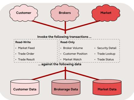
submits them to the system under test (SUT) and measures the rate of completed transactions being returned. To simplify the benchmark and focus on the core transactional performance, all application functions related to user-interface and display-functions have been excluded from the benchmark. The system under test is focused on portraying the components found on the sever side of a transaction monitor or application server.
