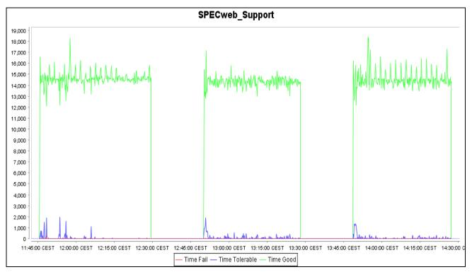
Figure 3: Three runs for the load profile Support and their QoS behaviour
