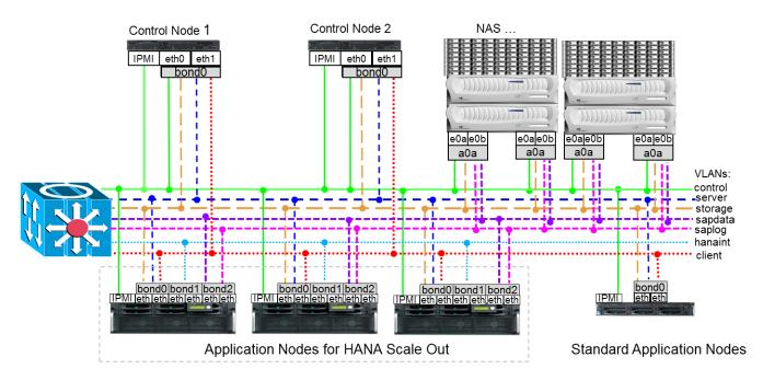
The bandwidth of the physical network has to be at least 1 Gbit/s for all components to handle intense data traffic. Selective network connections (for instance the connections from a FlexFrame NetApp NAS system or from a set of 10GbE-capable rack servers or blade servers (via switch blades) to the FlexFrame access layer switches) may be chosen as 10Gbit/s connections.
