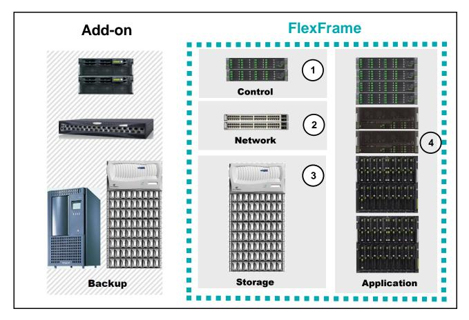
1. Control Nodes – the Control Center: Two PRIMERGY servers of type RX300/RX2540 with SUSE Linux Enterprise Server installed on local disks. Alternatively the Control Nodes can be realized as KVM virtual machines.
