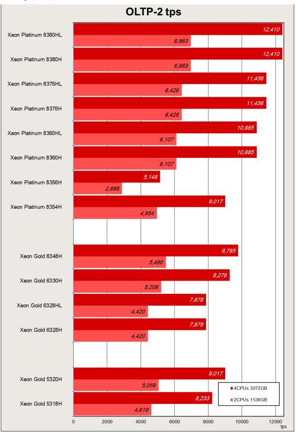
It is evident that a wide performance range is covered by the variety of released processors. If you compare the OLTP-2 value of the processor with the lowest performance (Xeon Platinum 8356H) with the value of the processor with the highest performance (Xeon Platinum 8380H) the OLTP-2 value increased by a factor of 2.4.
