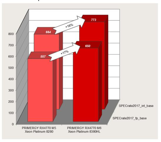
SPECrate2017: Comparison of PRIMERGY RX4770 M6 and PRIMERGY RX4770 M5
