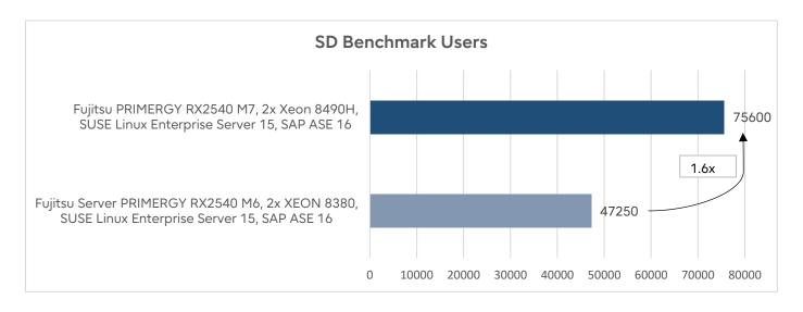
The 4th Generation Xeon Scalable Family (aka Sapphire Rapids) based RX2540 M7 with Intel Xeon Platinum 8490H delivers an improvement of 1.6x compared to the previous 3rd Generation Xeon Scalable Family (aka Ice Lake) based RX2540 M6 with Intel Xeon Platinum 8380 processor.
