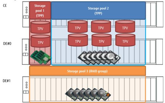
\*4: For the ETERNUS DX60 S5/S4 (3.5" type) and the ETERNUS AF250 S2, the above configuration is not available because only one drive enclosure (DE) maximum can be connected.
