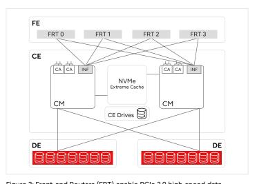
Figure 3: Front-end Routers (FRT) enable PCIe 3.0 high-speed data interchange between the controllers.
