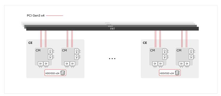
Figure 8: Schematic illustration of Controller Enclosures – all components in the enclosures are hot-pluggable.
