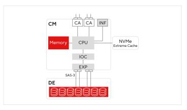
Figure 2: Controller Module (CM)
