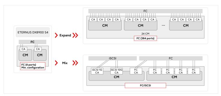
Figure 7: All types of Channel Adapters can be mixed on a Controller Module.
