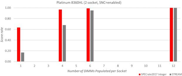
The processor model used for this test (and the later test of the same category) is a Xeon Platinum 8360HL. The DIMM type used is 32 GB 2Rx4 RDIMM.
