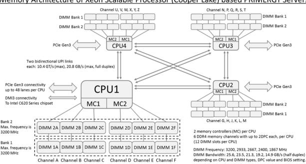
Memory Architecture of Xeon Scalable Processor (Cooper Lake) based PRIMERGY Servers
